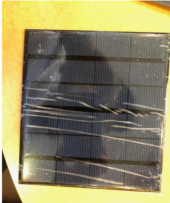
Figure 22: AMX3d 165mm x 135 mm 6.0V 600mA solar cell.
